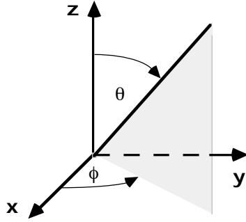
$$\begin{aligned}\sigma = & \sin^2 \theta (\sigma_{xx} \cos^2 \phi + \tau_{xy} \sin 2\phi + \sigma_{yy} \sin^2 \phi) + \sigma_{zz} \cos^2 \theta \\ & + \sin 2\theta (\tau_{yz} \sin \phi + \tau_{xz} \cos \phi)\end{aligned}$$
