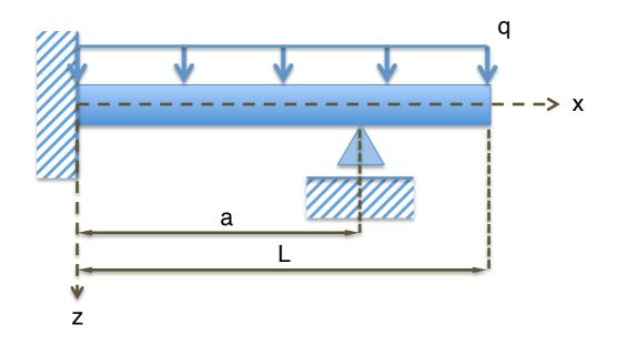
L = 8 m a = 5.92 m q = 0.25 kN/m E = 180 GPa  $I = 200 \text{ cm}^4$
